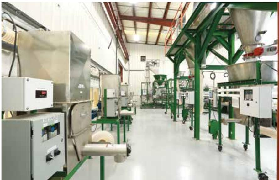
The supplier's newly renovated test center has a wide range of conveying and feeding equipment that can be arranged to mimic the customer's application.
