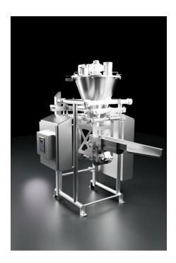
Thayer Scale's Hygienic Weigh Feeders (HWF), built in accordance with the design principles of 3-A, NSF and USDA, accurately measure the rate of flow of shredded cheese based on the direct measurement of mass and velocity variables. Cheese measurement takes place over a fixed length of the weigh feeder conveyor using a moving window average of measurements taken multiple times each second.
