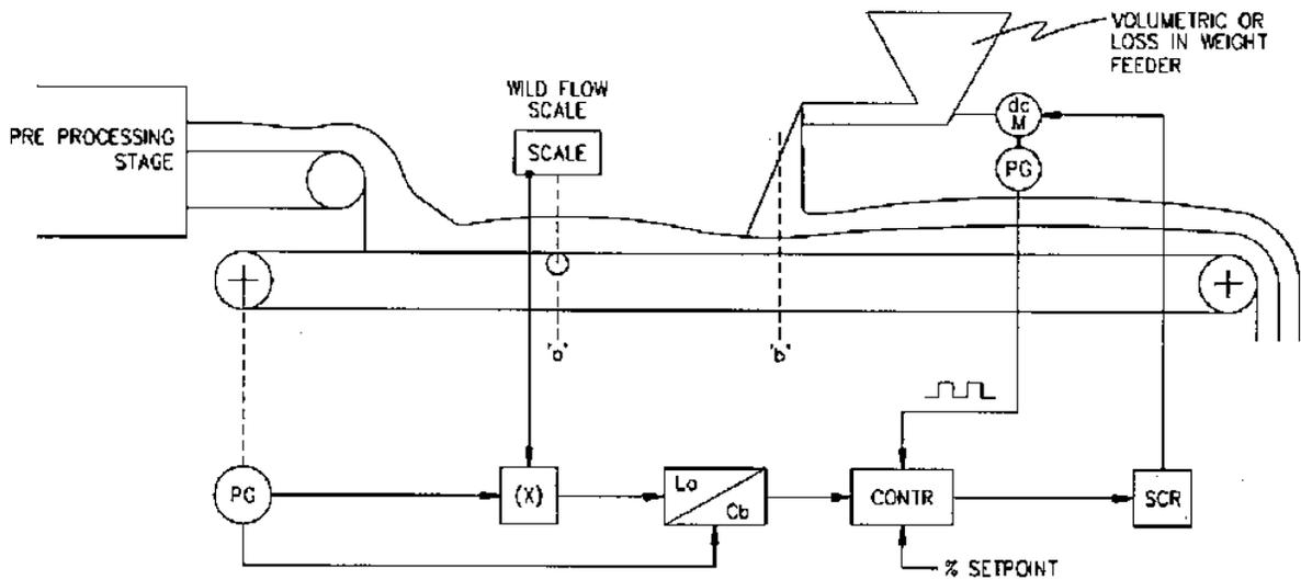
8. A Master Rate Setter station provides this system with a combined flow set point from which each ratio controller operates. Scale Location Compensation is used to delay the input demand to each downstream controller to assure complete "in-phase" blending along the entire length of the collecting conveyor. At the completion of the batch all feeders shut down in the reverse sequence, assuring blend accuracy throughout the entire run.
