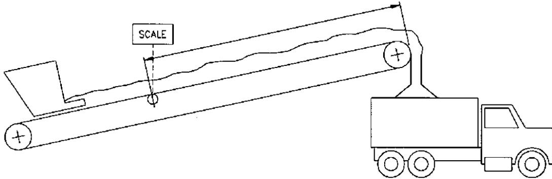
Note that conveyor scale is located near tail end, where belt tension is lowest, to assure best accuracy. Thus, all the material between scale and head pulley has been totalized but not delivered.
