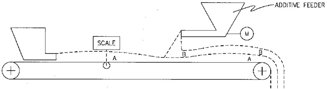
Note that heavy load at belt scale calls for proportionately greater additive feed, yet low loading at additive feeder's location requires an opposite response if instantaneous blend control is to be maintained. While these three examples meet different objectives, the basic problem that faces the process engineer in each case is the same:
