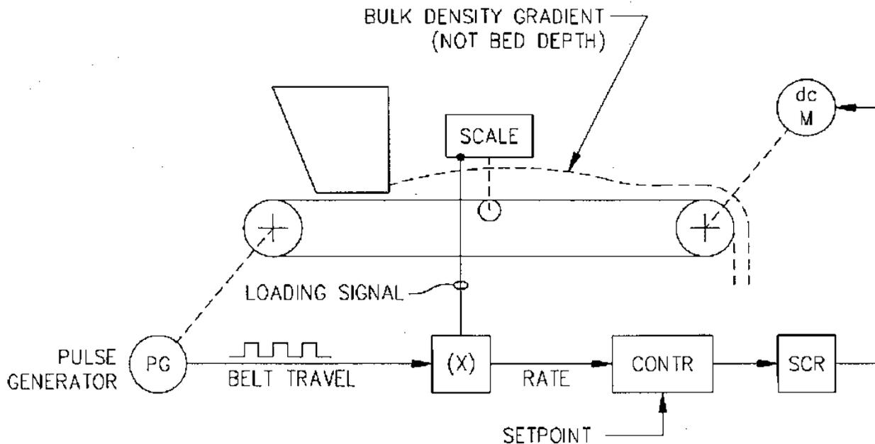
Note that heavy loading at scale calls for slower belt speed, yet light loading at head pulley requires opposite response if desired flow rate is to be achieved at the discharge.
