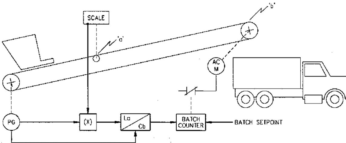
6. This system reports the measured variables discharging into a hostile environment while maintaining tight control of the weigh feeder that must be located a suitable distance away. The transport conveyor belting (steel belting in this example) may be chosen without restriction since the actual weighing is accomplished before the material is transferred to it.
