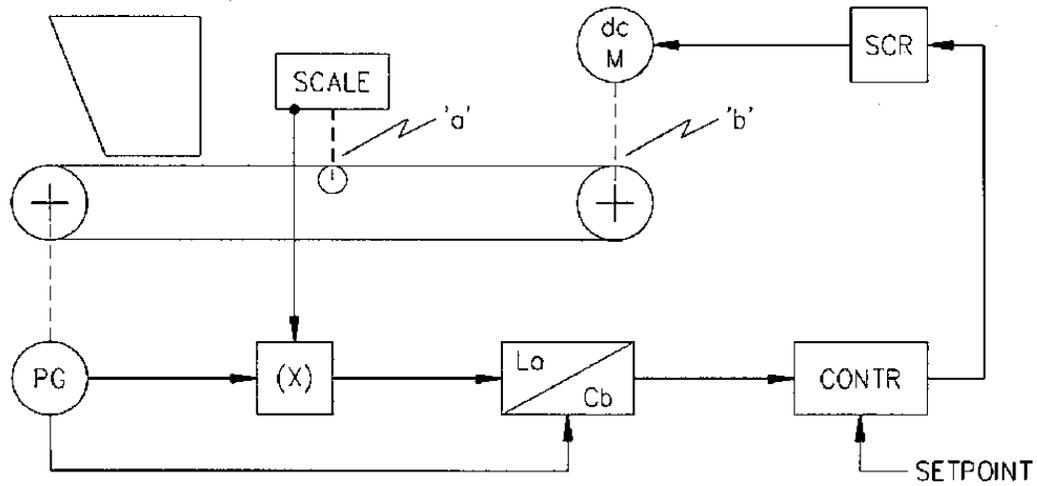
5. A system to measure the discharging quantity of flow from a load out conveyor. Scale should be located near material loading point from the standpoint of accuracy since lower belt tensions are conducive to high accuracy belt weighing. Of primary interest however is the quantity that has been delivered at the head pulley.
