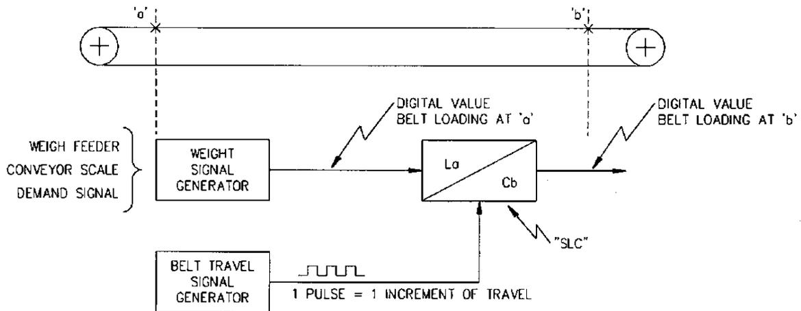
The "weight" signal may come from any continuous weighing or feeding device, or it may come from a demand signal generator (set point) transmitter.
