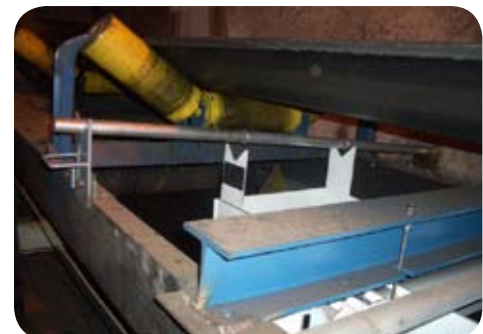
Belt Scale Test Weight and Manual Test Weight Lifter
