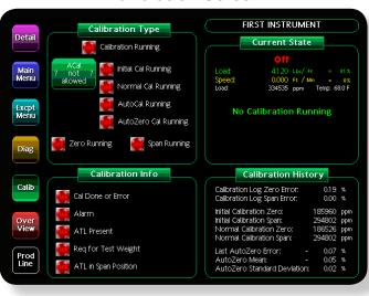
The user can follow calibrations preformed by the instrument here. Depending on the existence of an Automatic Test Weight Lifter (ATL or ATWL), and other menu entries, an Automatic calibration can be initiated here as well. If all conditions to run an AutoCal are not met, the button will show a "?". Tapping on this button will present the reasons the calibration cannot be performed.
