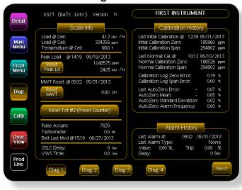
There are multiple diagnostic screens available for each instrument. The first shows the scale information as well as calibration and alarm histories.
