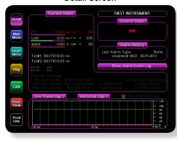
The Detail Screen show the most important information that the instrument provides. Specific information for Controllers (Belt and LWF) can be entered on this screen, such as RUN/OFF and Setpoint entry.
