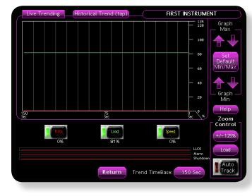
The Live Trend screen has advanced features that allow the user to zoom in and track a specific variable so it can be examined in finer detail. Controls for this are found on the right side of the screen.
