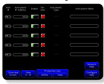
When the IP address has been entered, the TS-520 will check for the existence of that instrument on the network.
