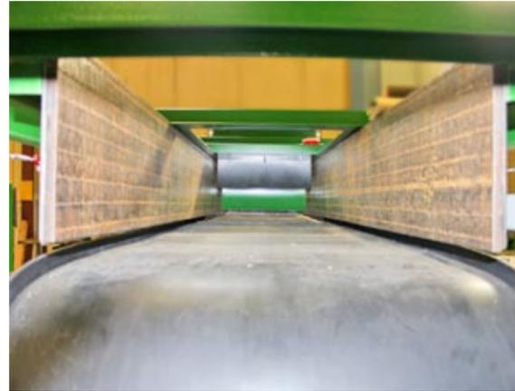
Installation of skirt boards along the entire length of the conveyor totally confines the material flow channel which helps control dust. Skirt boards are tapered and flared from the inlet to the discharge to prevent pinching of material between the skirt and the belt. The flare in the skirt boards also reduces friction and allows for lower motor horse power.
