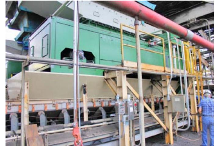
THAYER proposed a new scale design that included calibration test weights built right into the scale. During the calibration process the weigh belt integrator prompts the operator as to when the calibration test weight is to be applied to the scale. On the old system the test weights needed to be applied by hand. The new scale the weights are applied by pneumatic cylinders that lower and raise the weight onto the scale. This new design significantly reduced calibration time.
