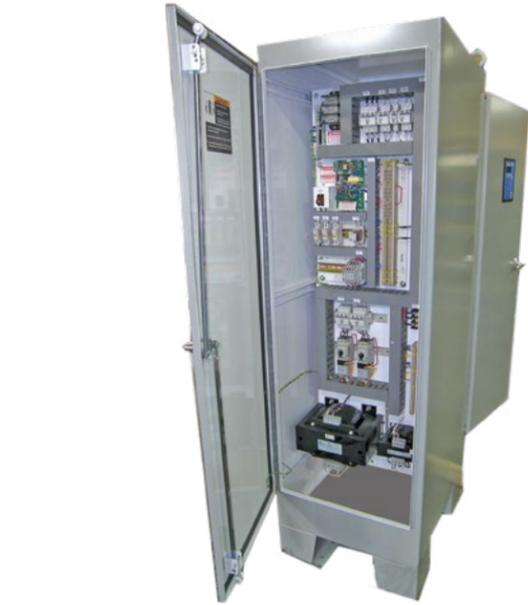
The system is controlled through a custom manufactured electrical panel. Thayer's Series 5200 Loss-In-Weight Controller monitors the output of the feeder and makes corrections in screw speed if required to maintain feed accuracy.
