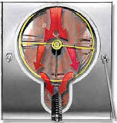
No Flood Design Stream of Material is deflected by the agitator bar, than curved sidewalls. Material velocity is reduced, controlling the tendency to aerate and flood.
