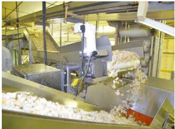
Thayer's Model SI was chosen because the SI uses the Thayer Force Measurement Suspension System that mechanically mass-counterbalances out the conveyor portion of the weigh belt. The scale only measures the weight of the croutons that pass over it. Additionally, it was important that the flow rate of the croutons be precisely regulated due to oven restrictions. Previously variations in product flow led to unevenly and overcooked croutons.
