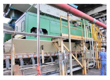
THAYER proposed a new scale design that included calibration test weights built right into the scale. During the calibration process the weigh belt integrator promps the operator as to when the calibration test weight is to be applied to the scale. On the old system the test weights needed to be applied by hand. The new scale the weights are applied by pneumatic cylinders that lower and raise the weight onto the scale. This new desin significantly reduced calibration time.
