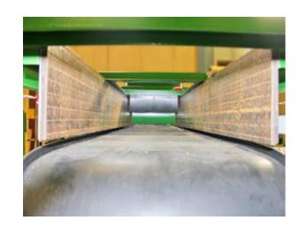
Installation of skirt boards along the entire length of the conveyor totally confines the material flow channel which helps control dust. Skirt boards are tapered and flared from the inlet to the discharge to prevent pinching of material between the skirt and the belt. The flare in the skirt boards also reduces friction and allows for lower motor horse power.
