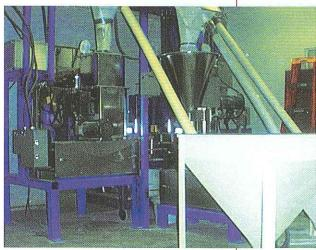
agglomerated and massed in the feeder, producing an unreliable discharge. In addition, the plant determined that the scaling system for the feeders did not provide sufficient resolution to accurately measure the material as it was
