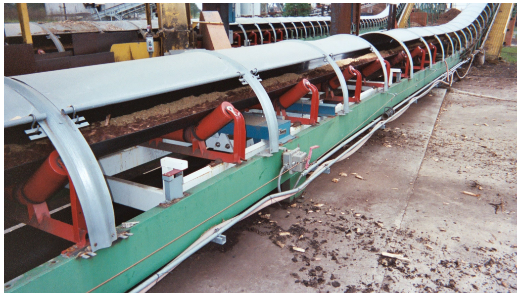
One of two conveyors with THAYER RF (rocking-flexure) belt scales
