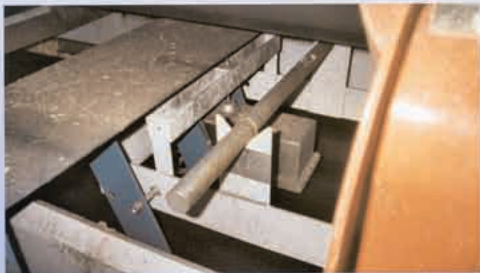
THAYER belt scales make use of small, bar-stock calibrating weights instead of heavy test weights, chains, or dummy signals.
