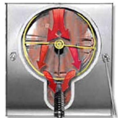
No Flood Design Stream of Material is deflected by the agitator bar, then curved sidewalls. Material velocity is reduced, controlling the tendency to aerate and flood.
