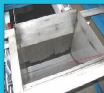
Chute is equipped with "flexible" gate to slow material velocity as it flows onto the belt surface
