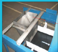
Material transfer chute mounted to conveyor frame
